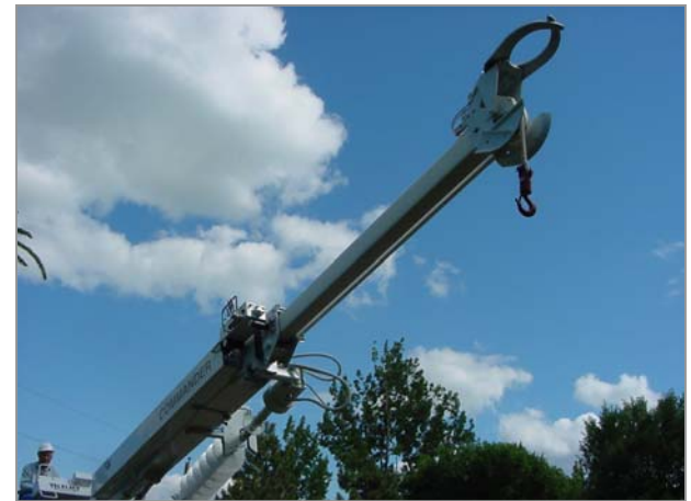
Pole Guides Transferred to Upper Boom
