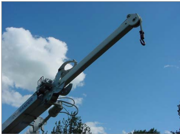
Pole Guides Pinned to Intermediate Boom
